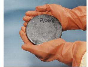
This gray metal is uranium. When made into nuclear fuel, it can power a nuclear reactor.
